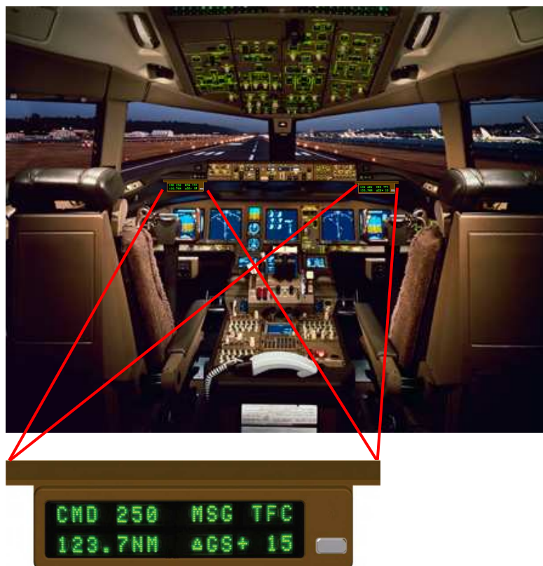
Figure 6-3 : Korry's ADS-B Guidance Display located under glareshield
