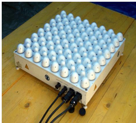
Figure 15: SFAS64 flat antenna array SODAR by Scintec consisting of 64 piezo-electric transducers (sound emitting and receiving units).
