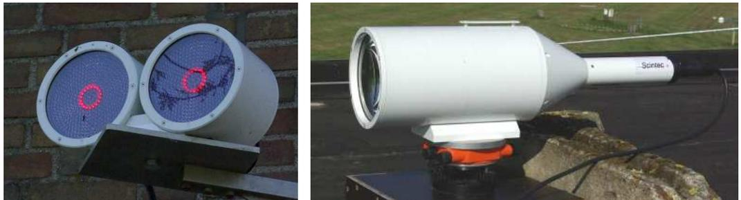
Figure 6: BLS900 scintillometer consisting of a dual aperture transmitter and a single aperture receiver.
