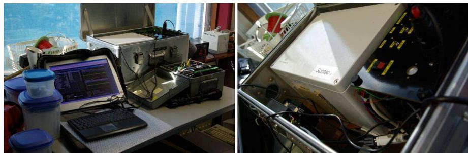
Figure 7: Processing unit and mini-pc built into a weather proof case. The portable screen and keyboard are only connected when accessing the unit in the field.
