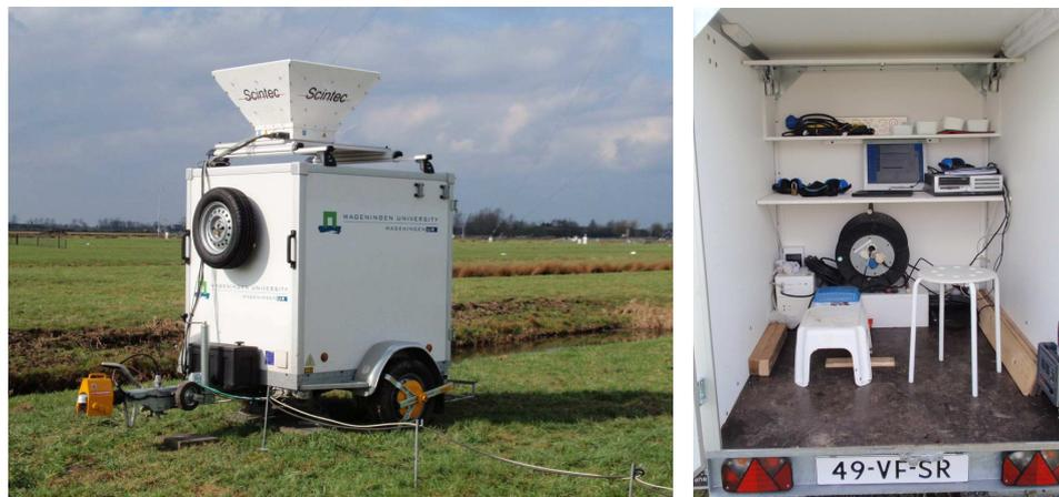
Figure 16: SODAR mobile platform developed during this project. The SODAR with small sound-screen is transported inside the trailer and is deployed on the roof of the trailer during an experiment. Processing units and computers are placed inside the trailer.
