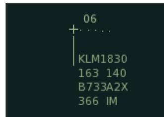
Figure 3. Track labels showing aircraft eligible for IM-operations (SPD#, left) and aircraft engaged in IM-operation (IM, right).
