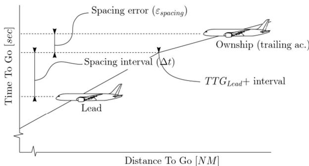
Figure 16: Time To Go spacing algorithm
