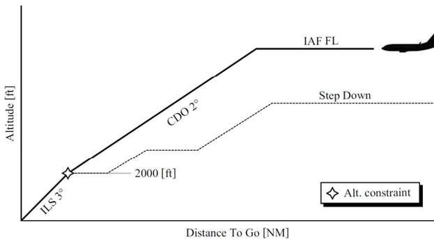
Figure 20: Vertical profile, the profiles are similar for each transition, the only difference is the IAF entry FL
