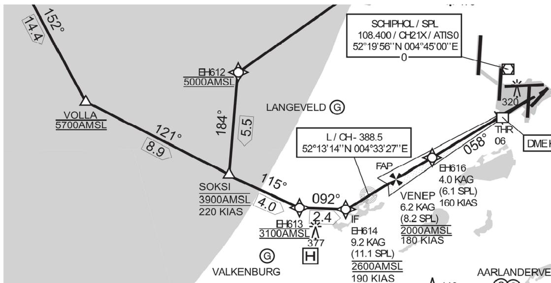
Figure 37 Detailed view of the SUGOL2X (from the left) and ARTIP2X (from the right) transitions to Runway 06
