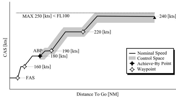
Figure 21: Speed profiles are equal for the four transitions, this is the nominal profile, ASTAR commanded speeds are within 10% of this profile
