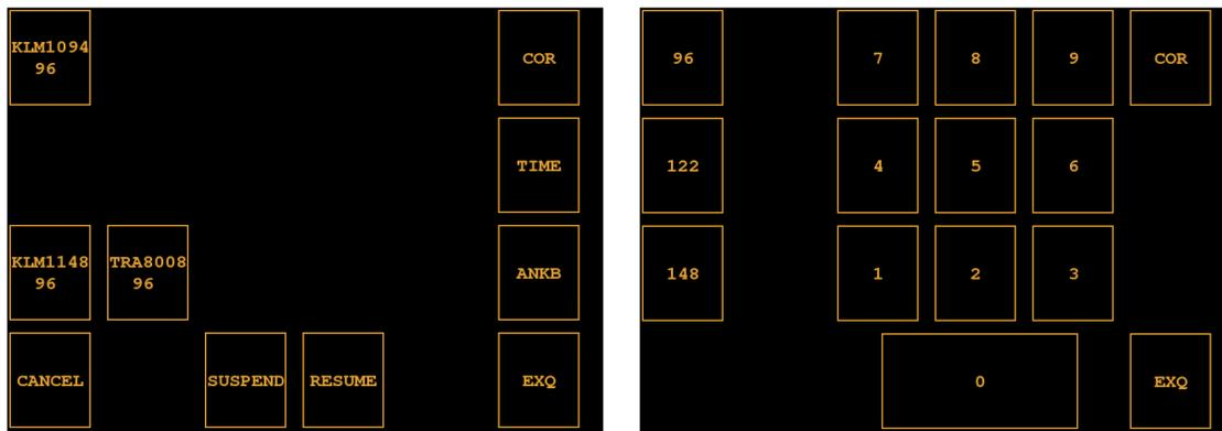
Figure 12. TID IM-sub-menus. Left shows the most logical target for IM-operations, followed by the second and third target possibilities, along with suspend and resume buttons. The right submenu shows the three standard time intervals.
