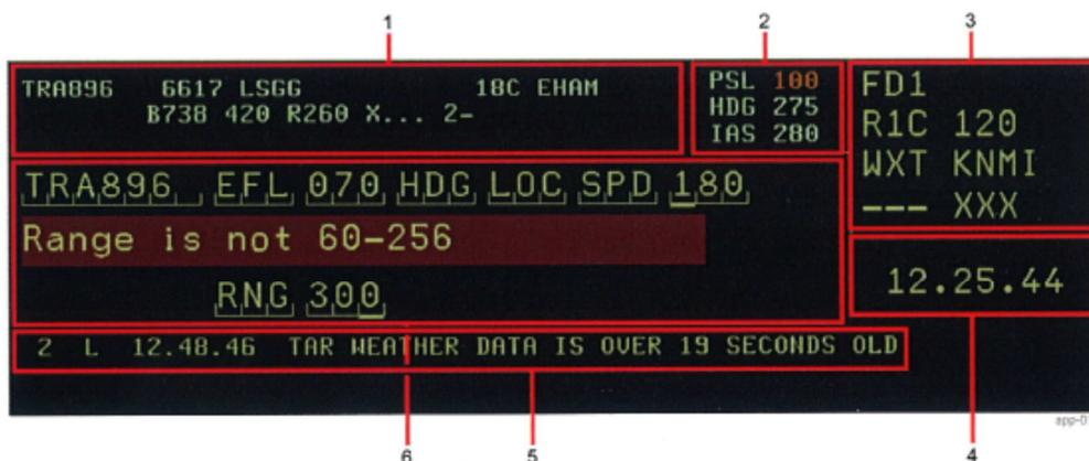
Figure 4. On-request line, displayed in the lower right corner of the plan view display.
