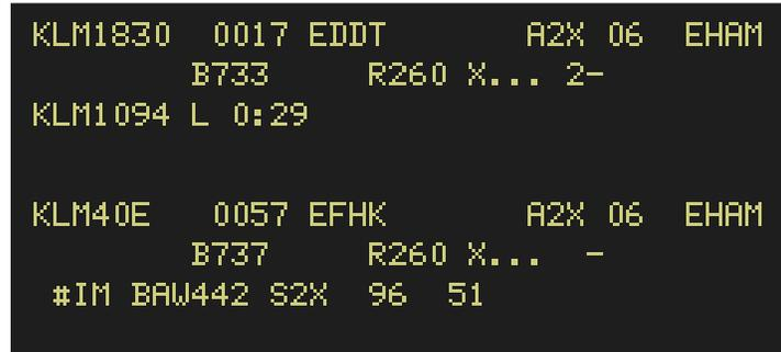
Figure 15. Augmented on-request line of radar display for non-IM and IM aircraft.
