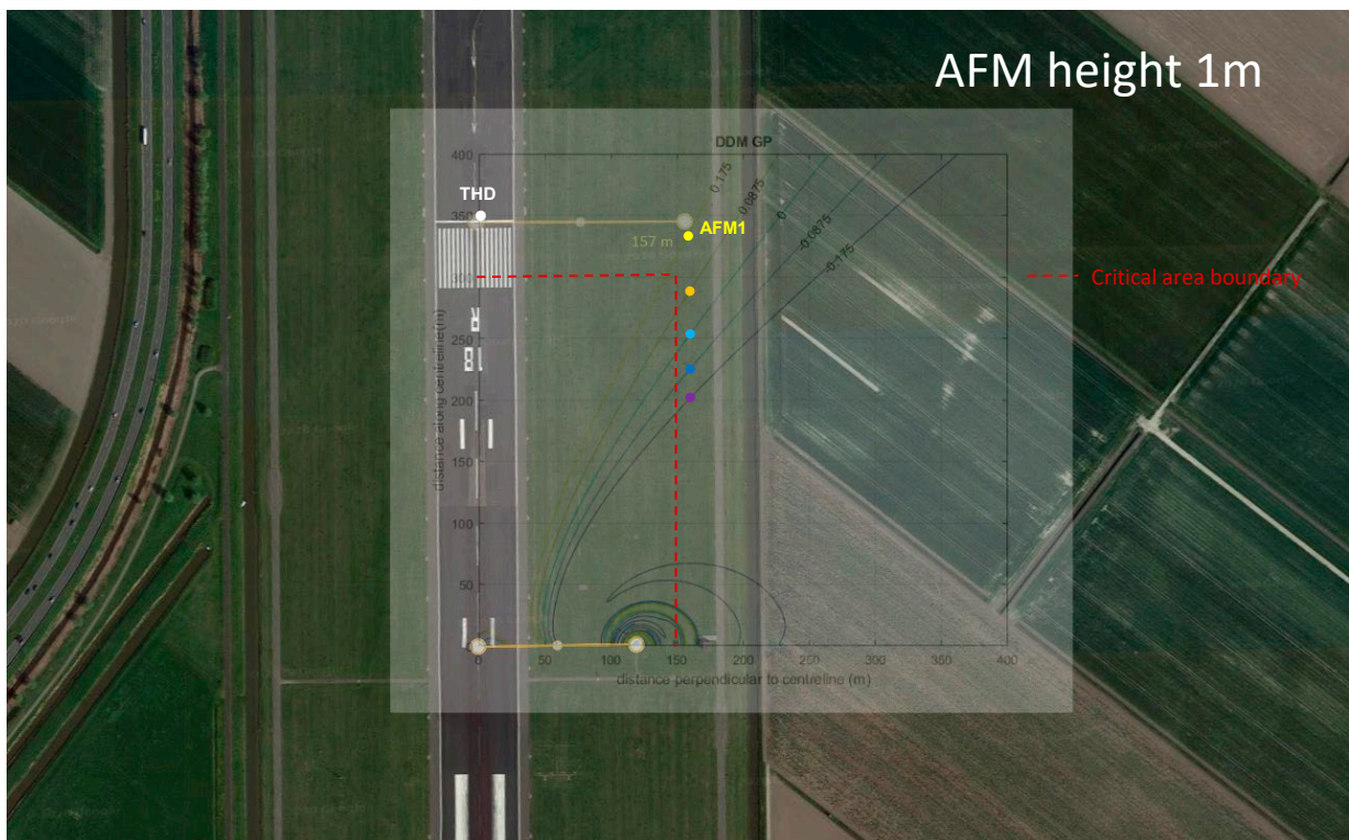
Figure 5: AFM locations near runway 18R indicated by the coloured dots just outside of the critical area
