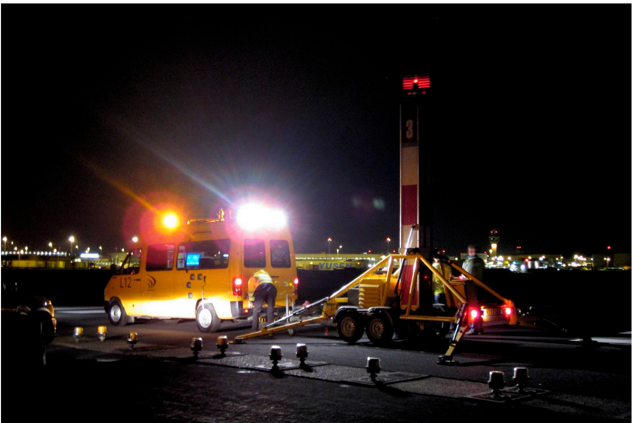
Figure 7: Preparation at Schiphol Airport of a ground measurement of the ILS GP signal in space
