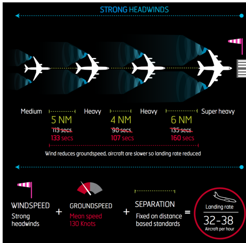
Figure 3.2: Aircraft Distance-Based Separation in strong headwind conditions. Values added for illustration purposes only [14]
