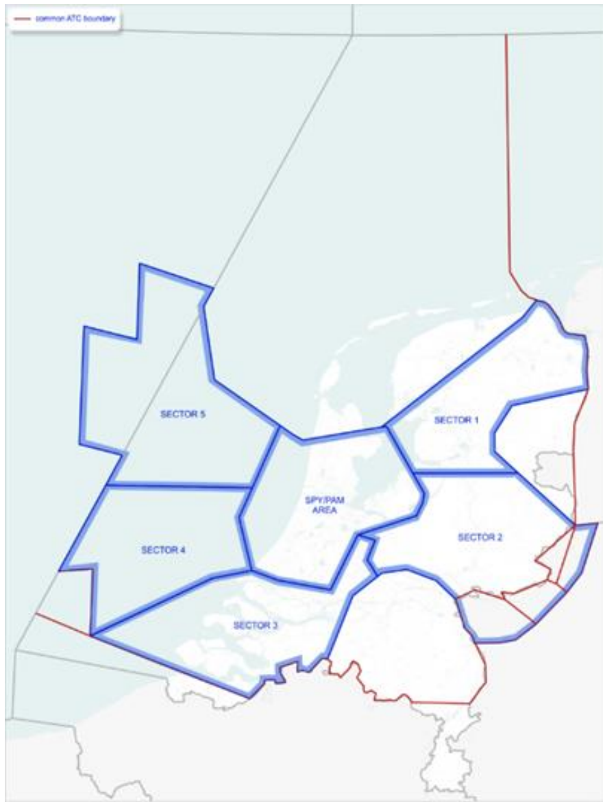
Figure 23: Sectors LVNL Area Control Centre according to Operational Manual (OM AMS ACC) ((Luchtverkeersleiding Nederland, n.d.-b)
