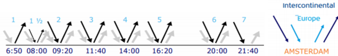
Figure 1: Seven wave hub system KLM at Amsterdam Airport Schiphol
