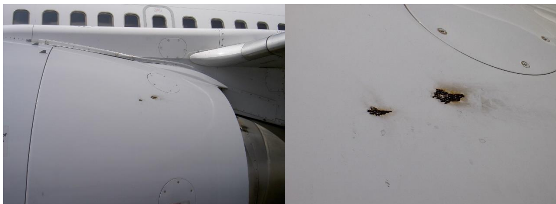
Figure 7 Two images of damage to the engine of an Airbus A380. The second (right) image is a close up of the first (left) image. Images supplied by an anonymous pilot.
